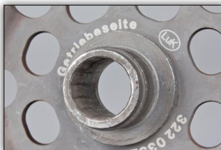
**Image 2:** Damaged spline profile
