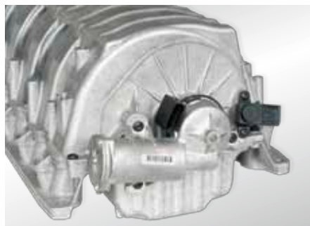
Drive module at the intake manifold
