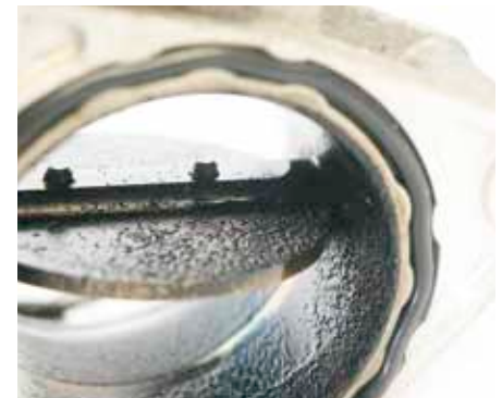
Regulating throttle suffering from oil contamination
