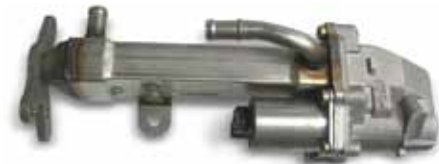
Fig. 1: EGR valve with EGR cooler
