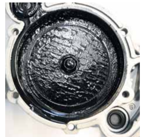
Fig. 3: Oil sludge in the vacuum pump of the VW Transporter results in rattling noises
